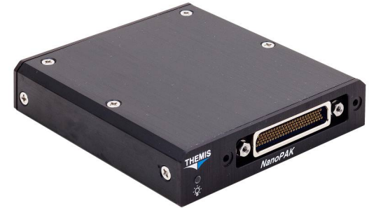
Atom or AMD-based NanoPAK 21 x 89 x 96 mm (HxWxD)
